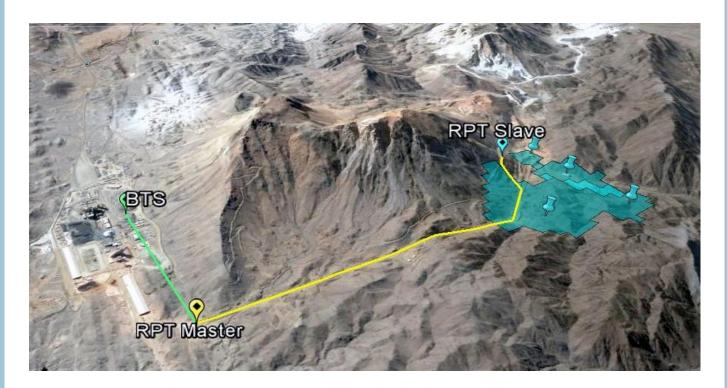
Typical RPT-9000DH applications include filling valleys and shadow areas that have large obstruction in the path such as a mountain or hill. With the Hybrid capability integrated into the master and slave units, two (2) strands of single mode fiber optic cable up to  $\sim 20$  Km is used to extend cellular signal to the area fill antennas.
